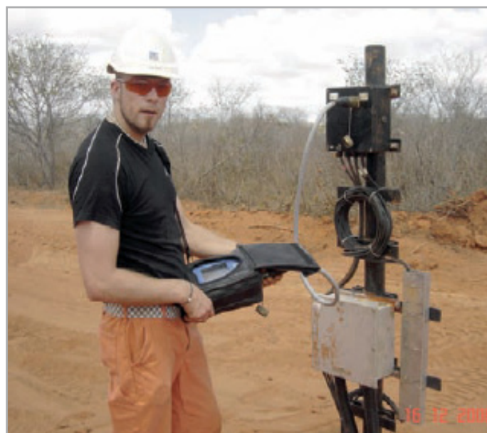
Operator collecting FSM-IT data using FSM-IT instrument at connection post for an underground pipeline.
